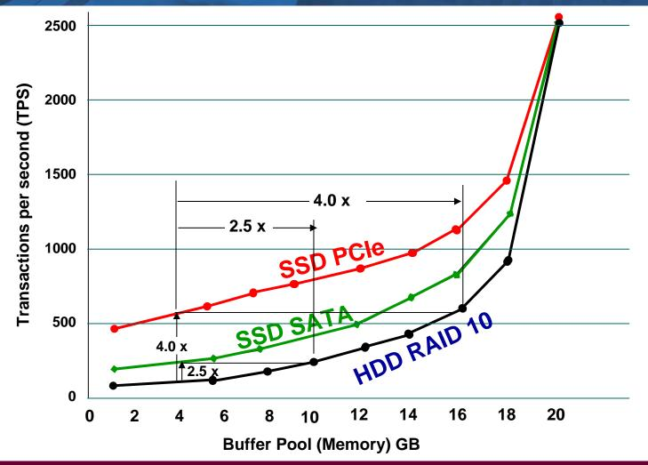
To achieve a certain TPS improvement, its cheaper to deploy SSD vs increased buffer memory (in GB costs) needed with using HDDs alone.
