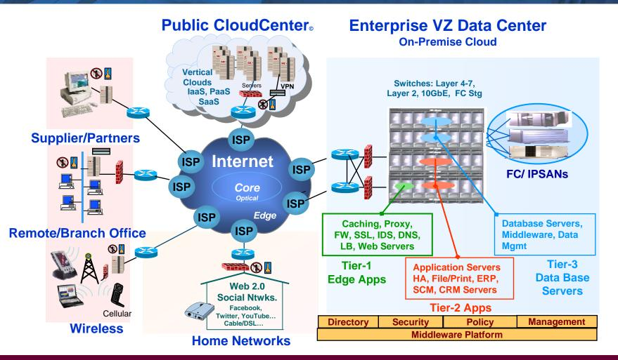
Request for data from a remote client to an enterprise data center crosses a myriad of systems and devices. Key is identifying bottlenecks & improving performance
