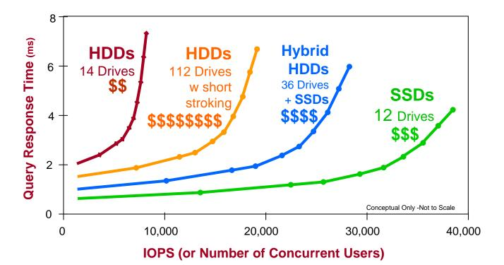
For a targeted query response time in DB & OLTP applications, many more concurrent users can be added cost-effectively when using SSDs or SSD + HDDs storage vs. adding more HDDs or short-stroking HDDs
